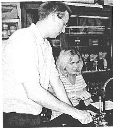
Mr. Doug Vogel adjusts the gas valve as Sarah Flannagan uses the flint stricker to light the bunsen burner
